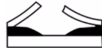
Over Etch and Resist Lifting
